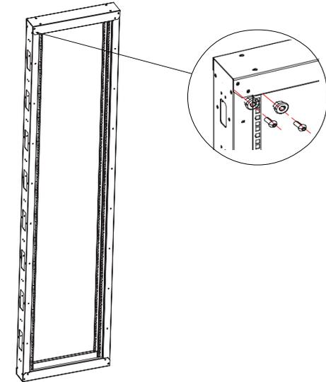
Step 1: Assembly vertical rails and horizontal beams to form the frame with 16 sets M6\*12 screws and M6 flange nuts.
