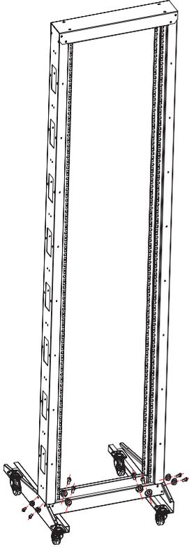
Step 3: Assembly the frame and plinth by 8 sets M6\*12 screws and M6 flange nuts.
