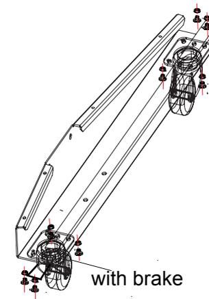
Step 2: Assembly the castors on the Plinths by 16 sets M6\*12 screws and M6 flange nuts.
