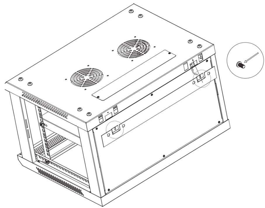
(5) Assembly the mounting bracket by 2pcs M4\*8 self- tapping screws.
