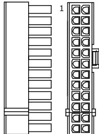
Pins 11/ 12/ 23/ 24 are made as separate jacks.
