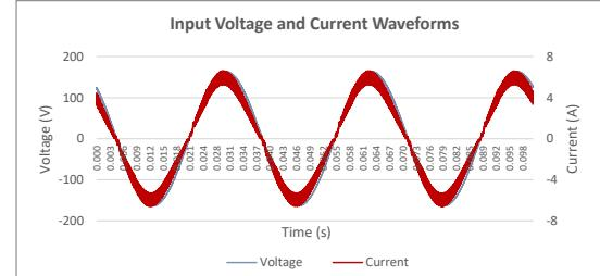
Input AC Current Waveform (ITHD = 4.53%, 50% Load)
