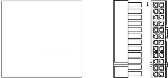
Pins 11/ 12/ 23/ 24 are made as separate jacks. It can be swung away in case of using older Mainboards.
