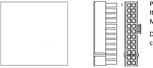
Pins 11/ 12/ 23/ 24 are made as separate jacks. It can be swung away in case of using older Mainboards.
