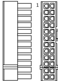
Pins 11/ 12/ 23/ 24 are made as separate jacks. It can be swung away in case of using older Mainboards.
