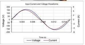
Input AC Current Waveform (ITHD = 5.52%, 50% Load)
