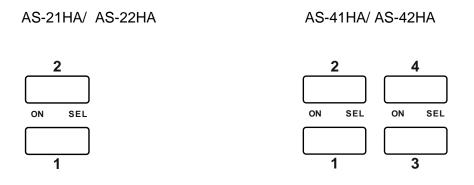
The switches at the front of the device are control buttons as well as LED indicators.
