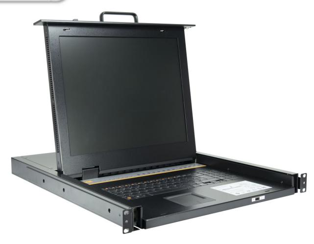
The **KVM-1708 LED** is a professional 8-Port KVM-Console with integrated extractable keyboard and 17" LED monitor. The **KVM-1708 LED** finds it's usage in server racks to switch and manage several installed servers.
