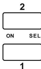
The switches at the front of the device are control buttons as well as LED indicators.
