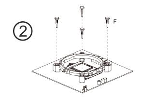
Put the bracket D onto the socket and fix it with pins F.
