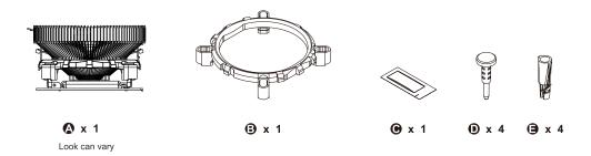
The included socket adapter B is for Intel-Socket 775/ 1150/ 1151/ 1155/ 1156/ 1366 mounting. There's no adapter necessary for mounting on AMD-Socket FM2+/ FM2/ FM1/ AM4/ AM3+/ AM3/ AM2+/ AM2. This cooler won't fit on any other socket as those mentioned before.
