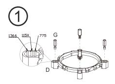
Press the transparent plastic adapter G, depending your socket, into the bracket D
