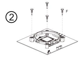
Place the mounting D onto the socket and fix it with pins F.
