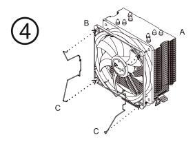
Fix the fan B with clamps C onto the cooler.
