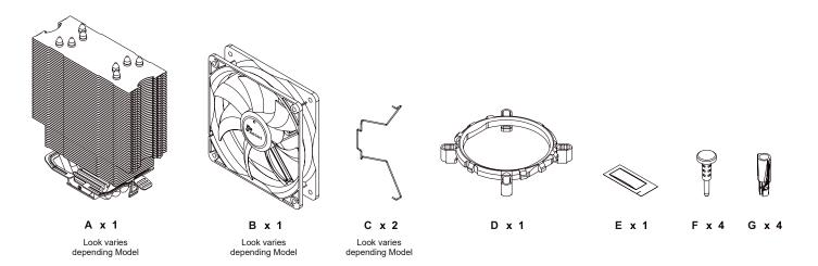
The included Adapter D provides the mounting on Intel socket 775/ 1150/ 1151/ 1155/ 1156/ 1366. For mounting on AMD socket FM2+/ FM2/ FM1/ AM4/ AM3+/ AM3/ AM2+/ AM2 is the adapter not necessary. Only mounting on the mentioned sockets is possible.
