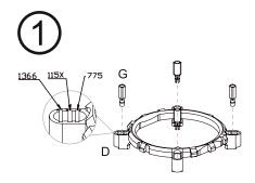
Push the clear plastic adapter G into the mounting D, depending your socket.
